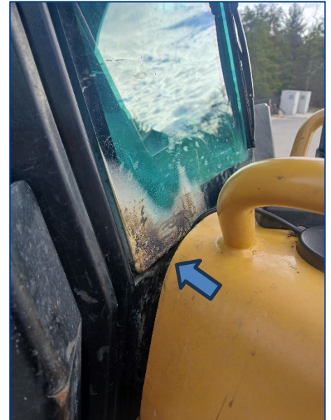
Fire damage on Dozer 252's windshield. Arrow points to the small gap between hood cowl and windshield that can collect debris.
